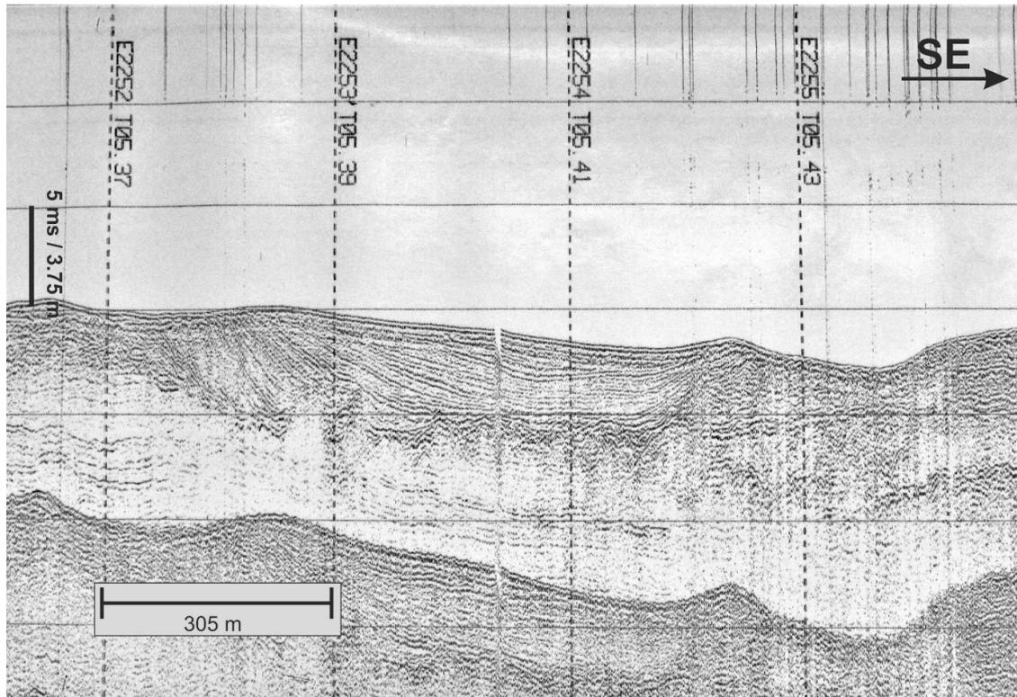
Figure 11 Channel seen to the north-west of the main study area, line C29 (see Figure 6 for location in the wider context)
