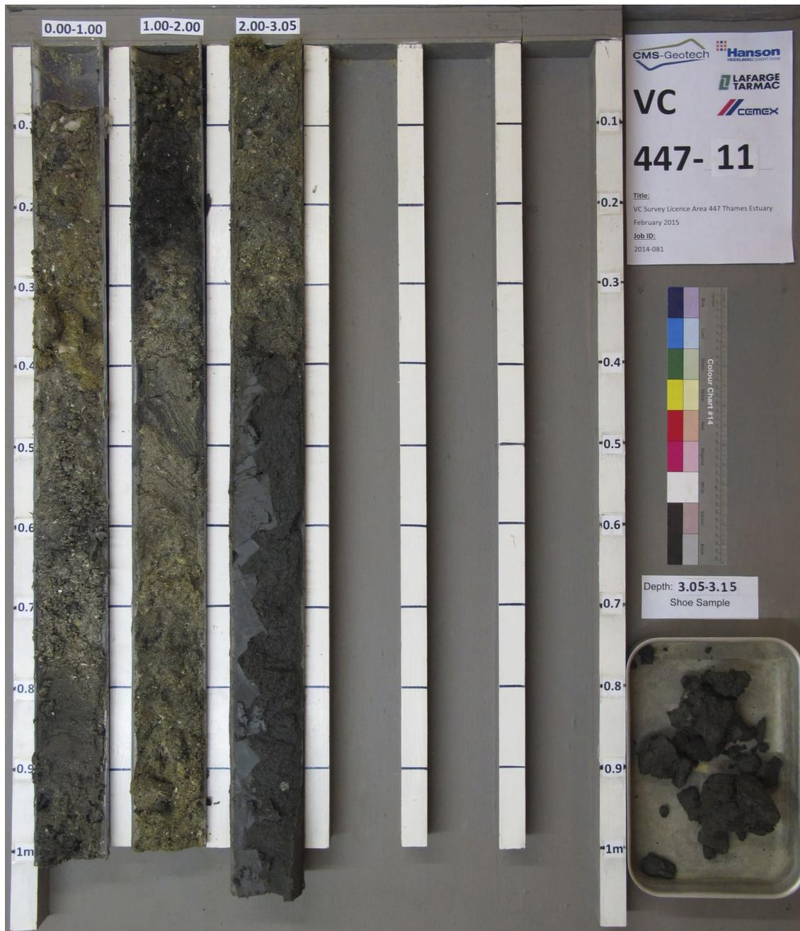
Figure 20 Photograph of vibrocore VC11
