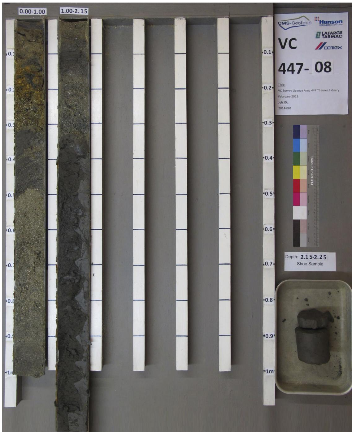
Figure 19 Photograph of vibrocore VC08
