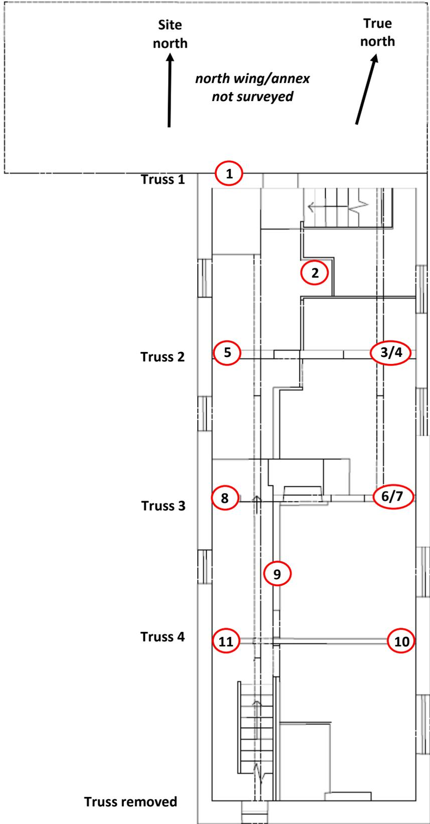
Figure 3a: Plan at first-floor level to show the locations of the sampled timbers (after Rebecca Lane 2021)
