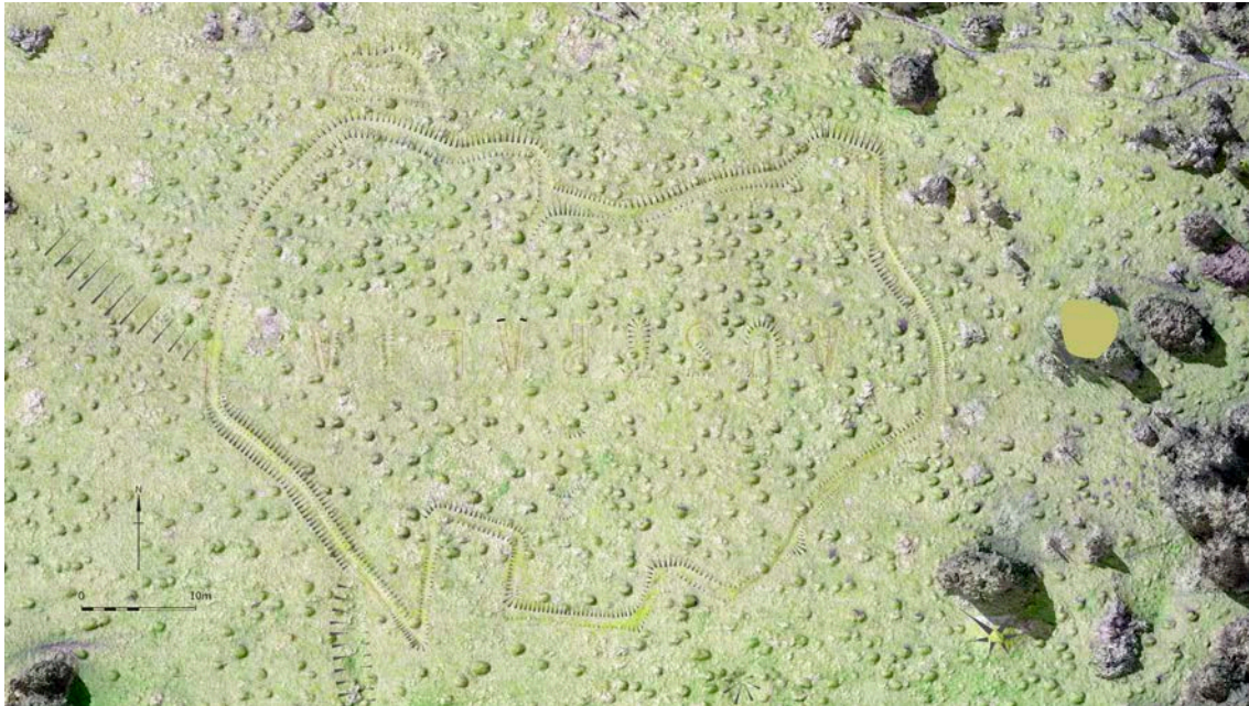
Figure 11: The hachured analytical earthwork survey shown against an orthophotograph generated from the SUA survey data, with the hillshade lit from the northwest and exaggerated [x2] to bring out the subtle detail. The numerous lumps are anthills.
