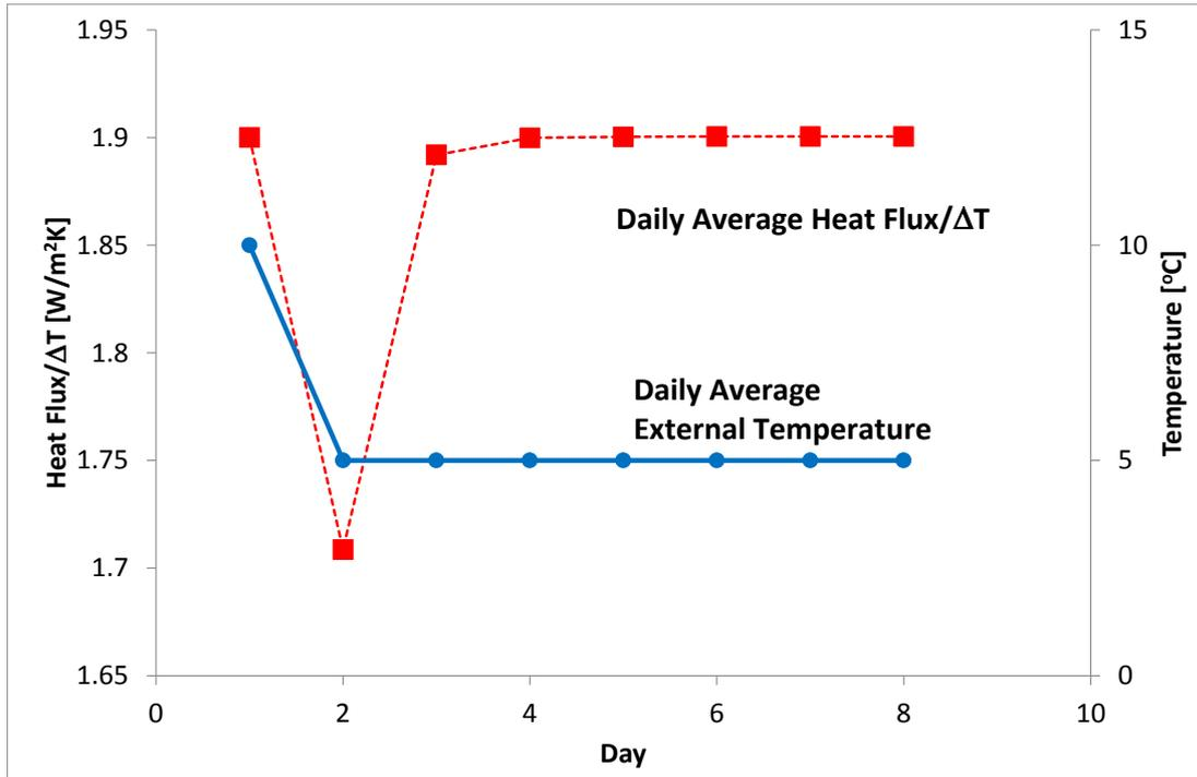
Figure A5: Demonstration of the effect of the step change in external temperature on the daily average value of the heat flux/ $\Delta T$ .
