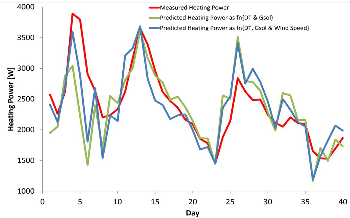
Figure A13: Before-intervention case. Measured and predicted heating power using (a)  $\Delta T$  and  $G_{sol}$  as the independent variables (Equation A1) and (b)  $\Delta T$ ,  $G_{sol}$  and wind speed (Equation A4).
