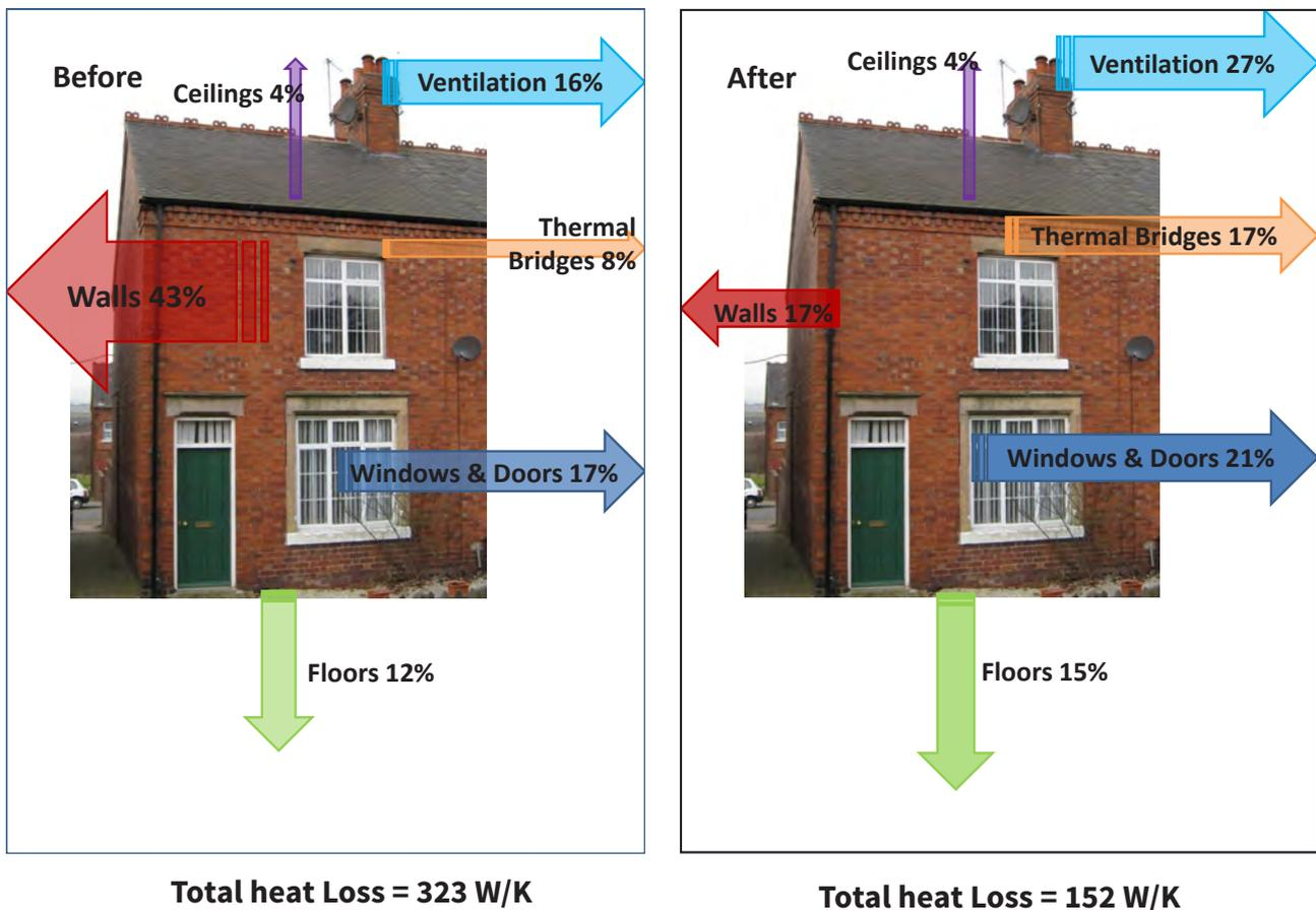
Figure 12: The proportions of heat loss through the building elements, thermal bridges and ventilation before (left) and after (right) the interventions.
