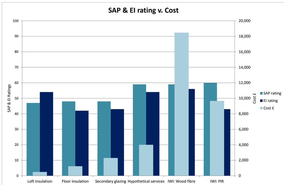
Figure 34: A comparison of SAP & EI ratings against cost of each measure
