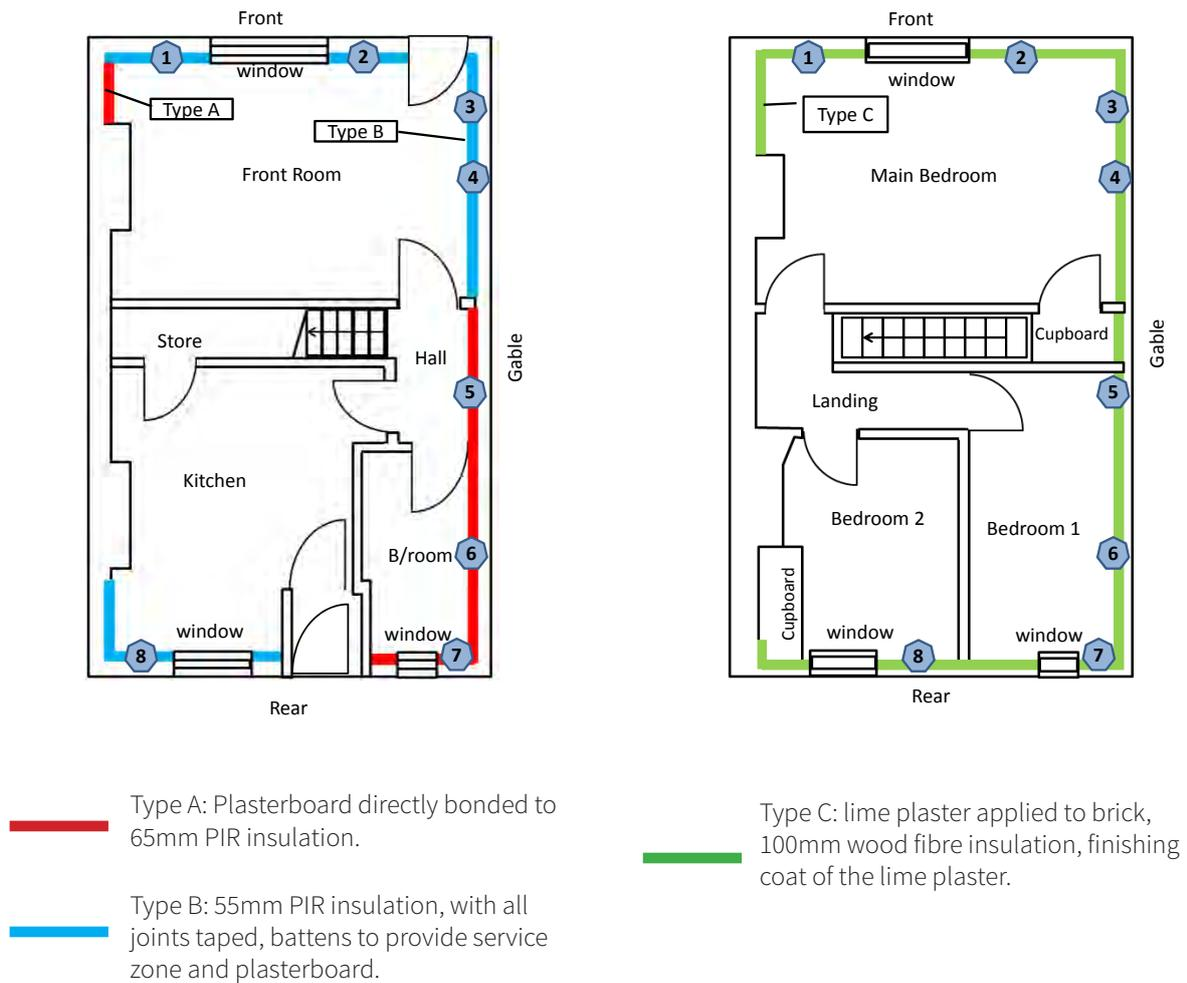
Figure 4: Location of the two internal wall insulation systems – left: ground floor with PIR; right: first floor with wood fibre system.
