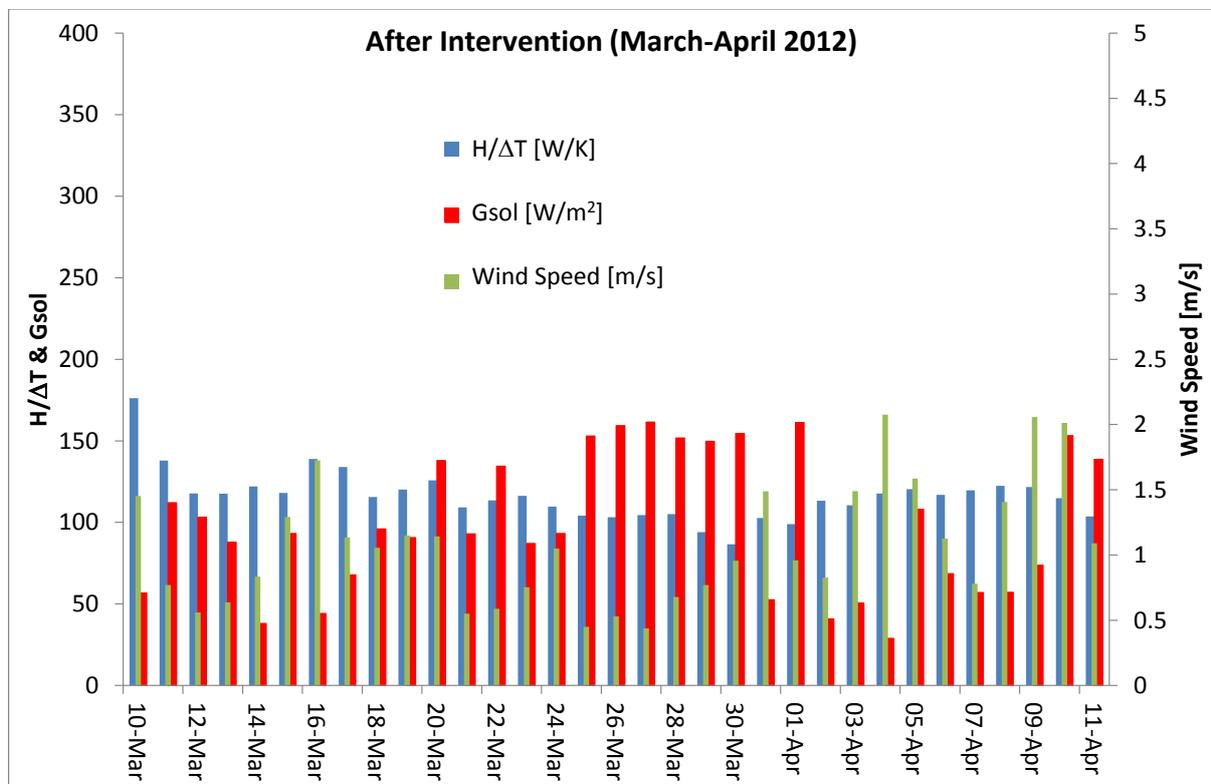
Figure 14: After Intervention. The daily average values of H/ΔT, Gsol and wind speed during the co-heating test.
