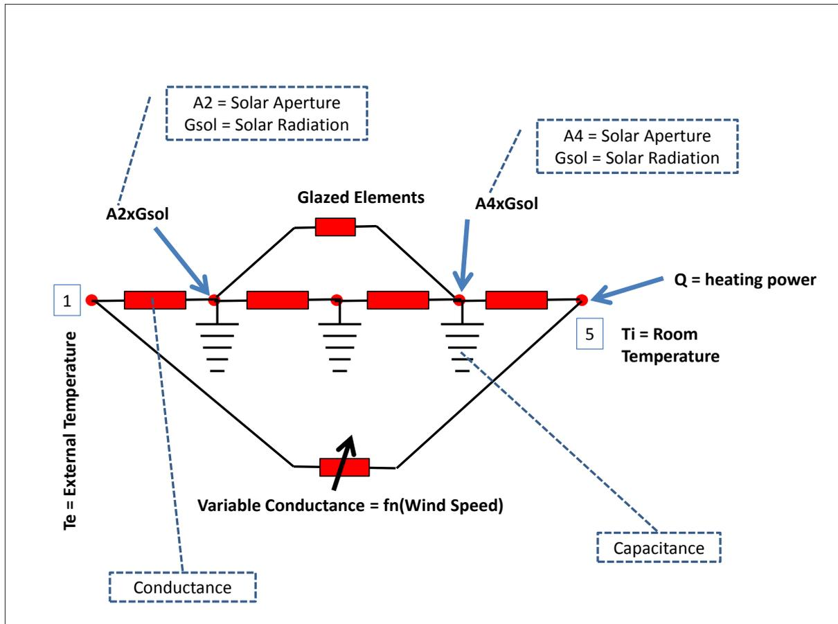
Figure A15: House modelled as a network of conductances and capacitances.
