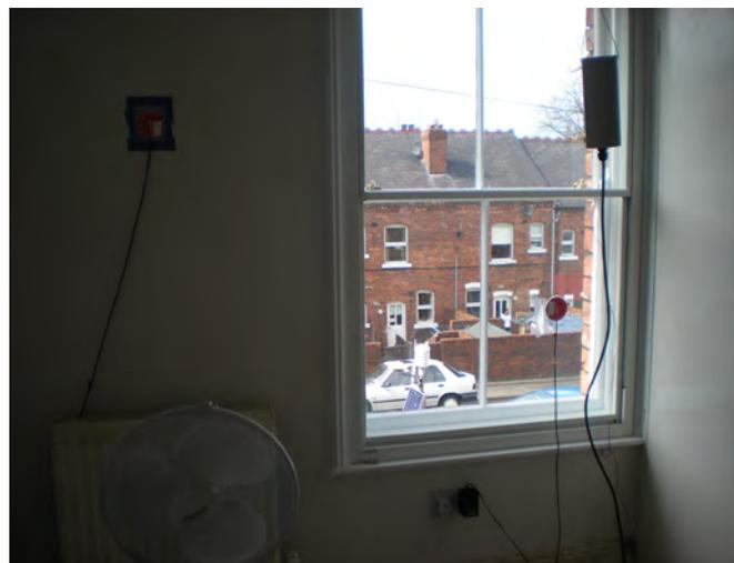
Figure 6: In situ U-value measurement on secondary glazing and adjacent wall in bedroom 2.
