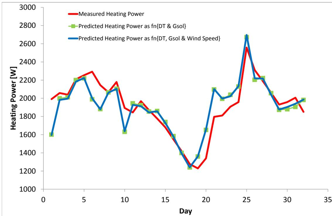
Figure A14: Post-intervention case. Measured and predicted heating power using (a)  $\Delta T$  and  $G_{sol}$  as the independent variables (Equation A1) and (b)  $\Delta T$ ,  $G_{sol}$  and wind speed (Equation A4). Note: the line for the two predictions of heating power are effectively co-incident.
