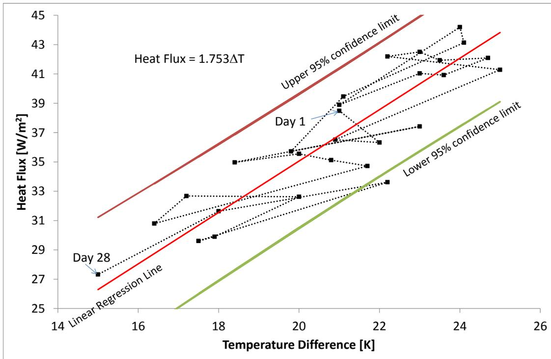
Figure A6: Daily average heat flux vs. temperature difference for simulated data using varying external temperature with 9" brick wall. The linear regression line, the slope of which gives the U-value, and the confidence limits.
