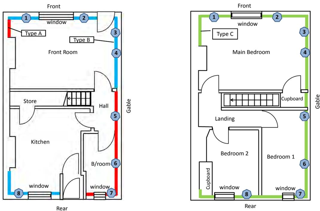
Figure 27: Plan of the monitoring locations with two sensors in each location positioned at low and high level
