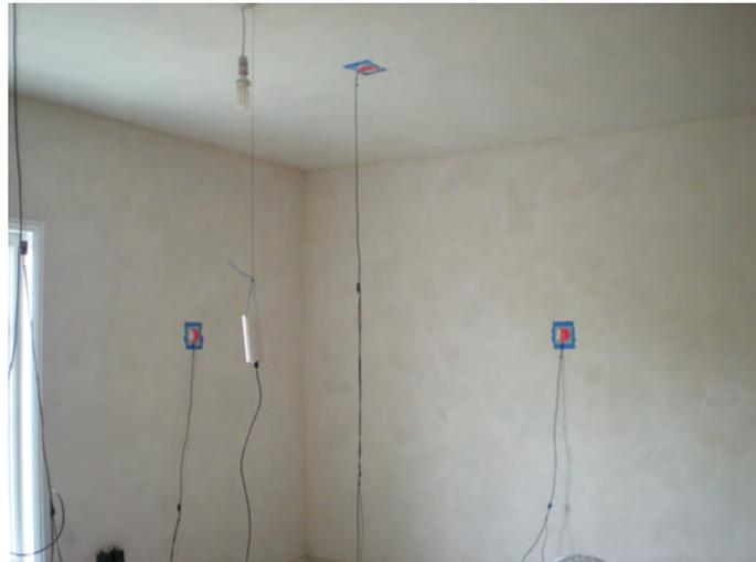
Figure 5: In situ U-value measurements in main bedroom: front elevation, gable wall and ceiling.
