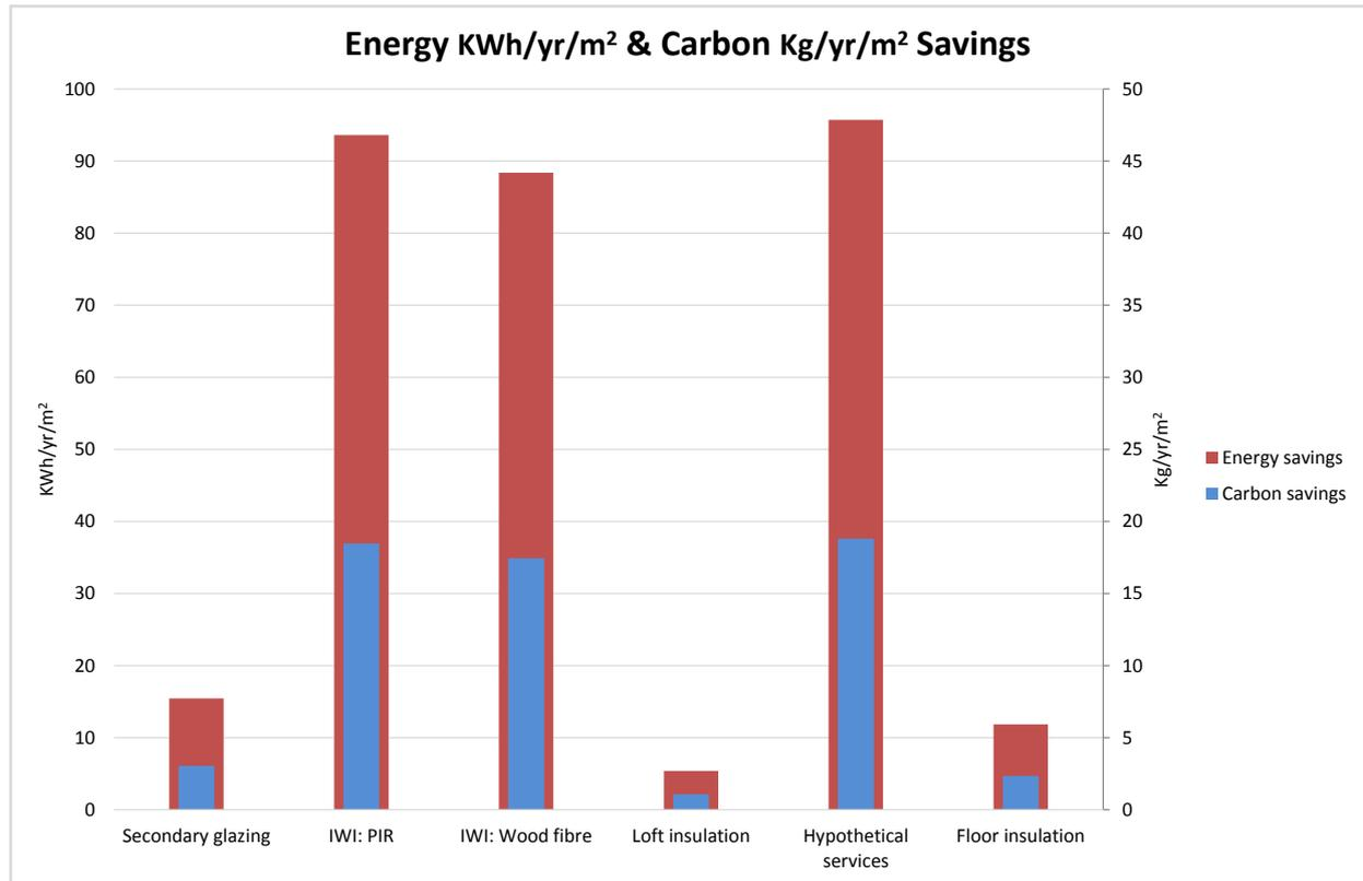
Figure 35: Energy and carbon savings for each measure
