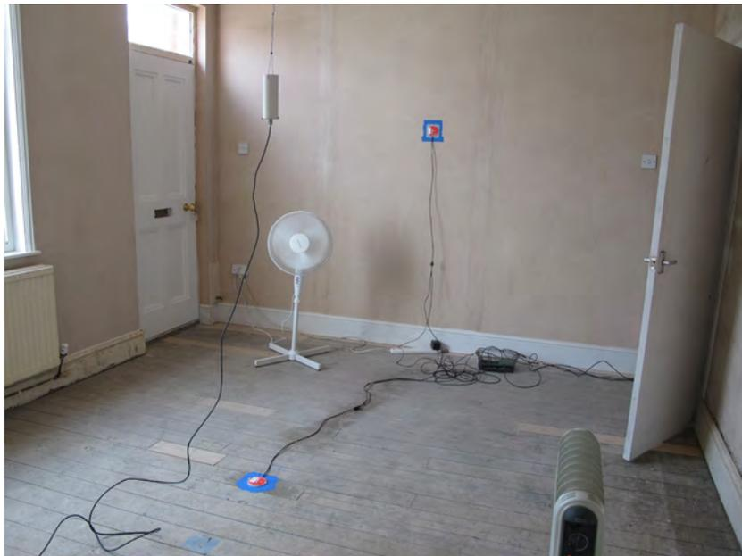
Figure 26: Co-heating test set-up
