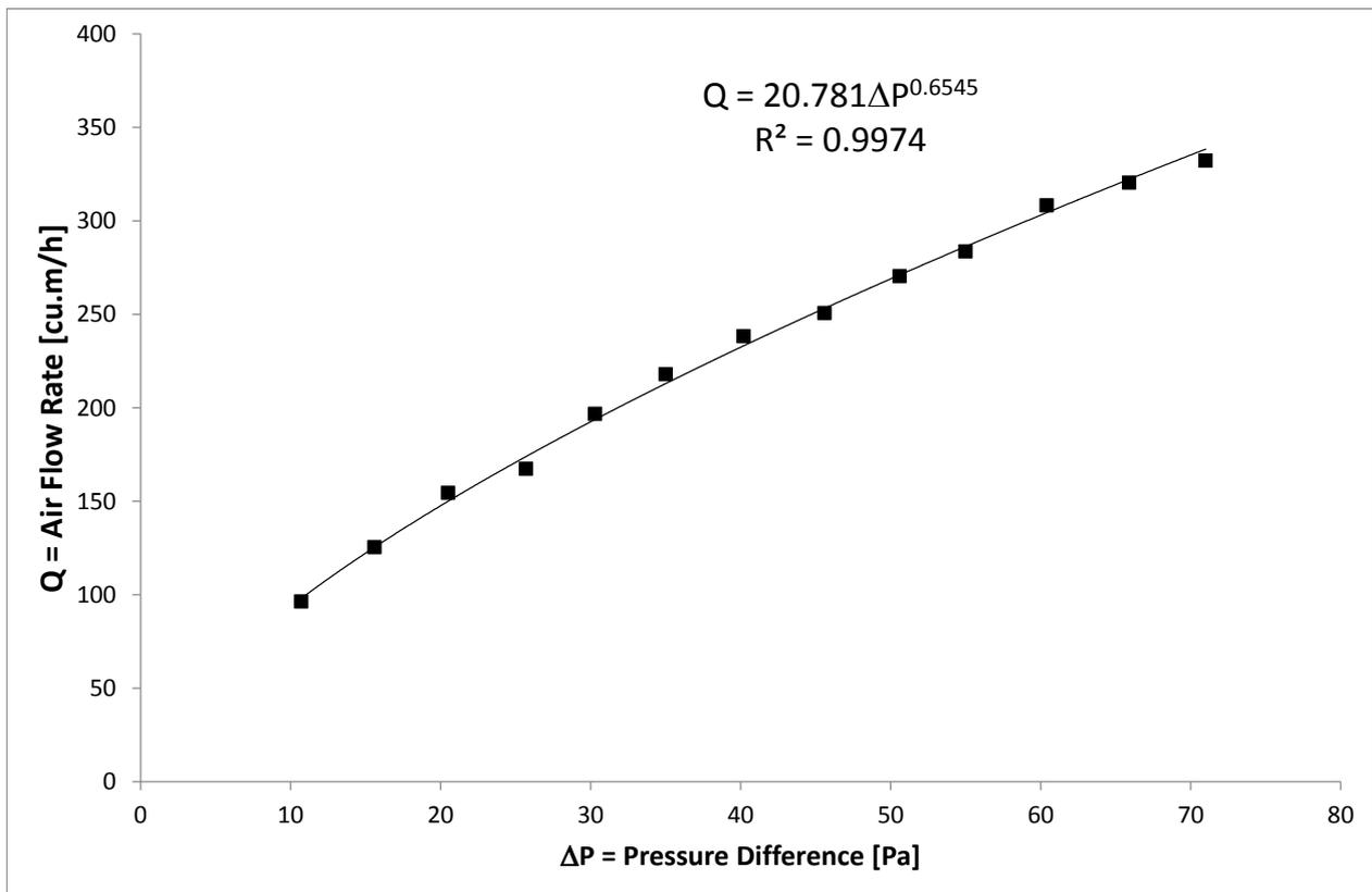
Figure 8: Example of building pressurisation test data with power law curve fit
