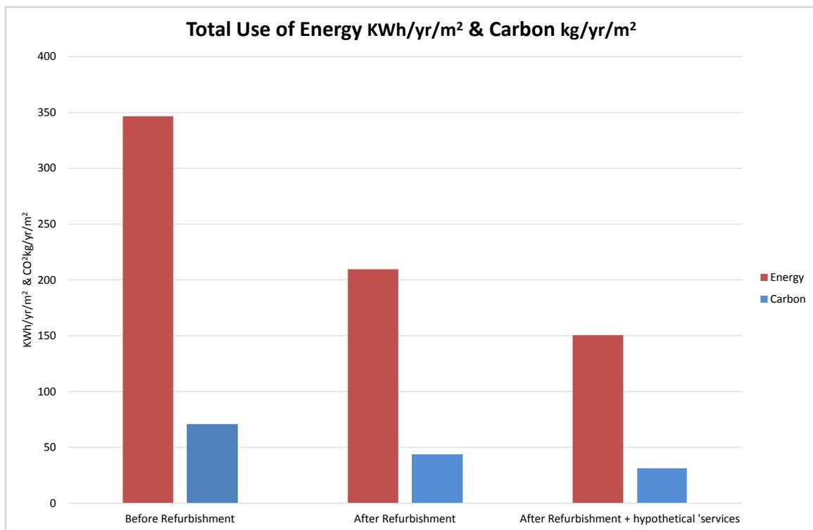
Figure 32: Total energy and carbon use before and after refurbishment, including installation of hypothetical services
