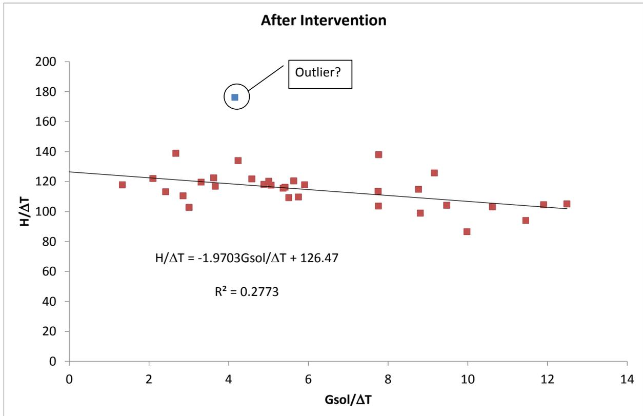
Figure A11: After Intervention.  $H/\Delta T$  vs.  $G_{sol}/\Delta T$  plot for the daily average values from the co-heating test. The linear regression fit for all the data without the outlier is shown.
