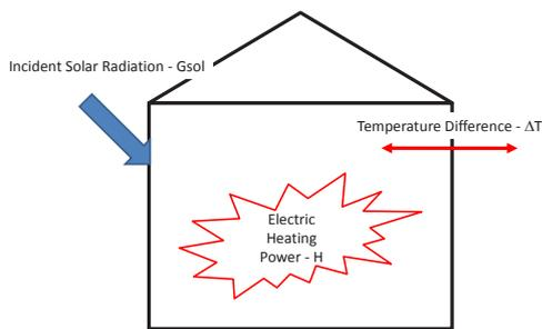
Figure A1: Schematic diagram of main parameters for analysis of co-heating test data using simplified analysis
