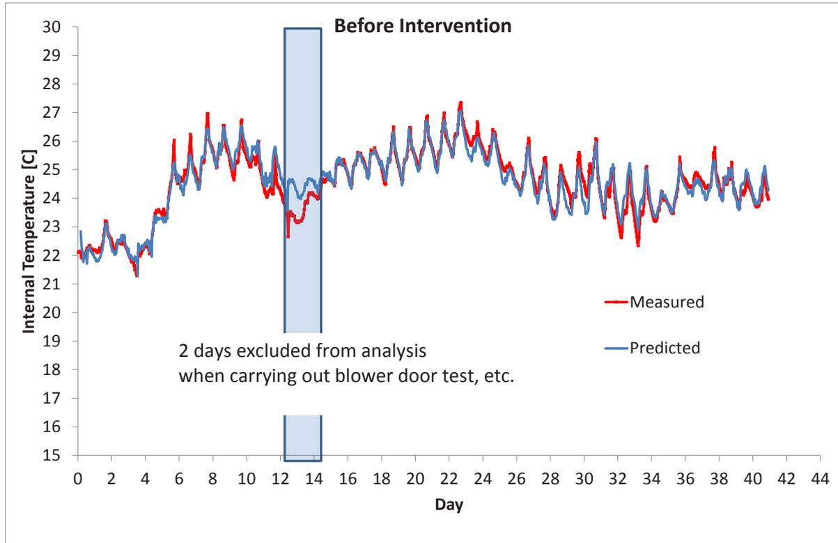
Figure A16: The predicted and measured output variable (average room temperature in the house)
