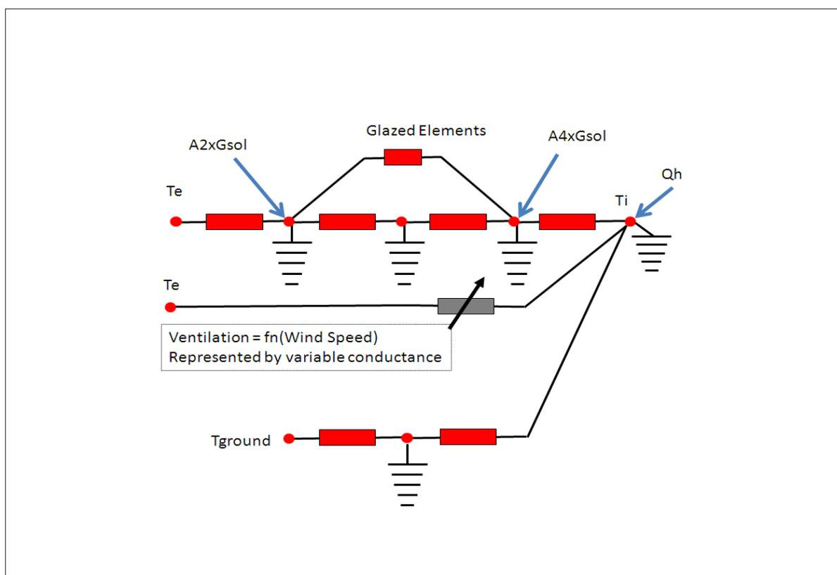
Figure A7: House modelled as a network of conductances and capacitances.
