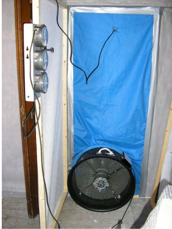
Figure 7: Blower door assembly for building pressurisation test.
