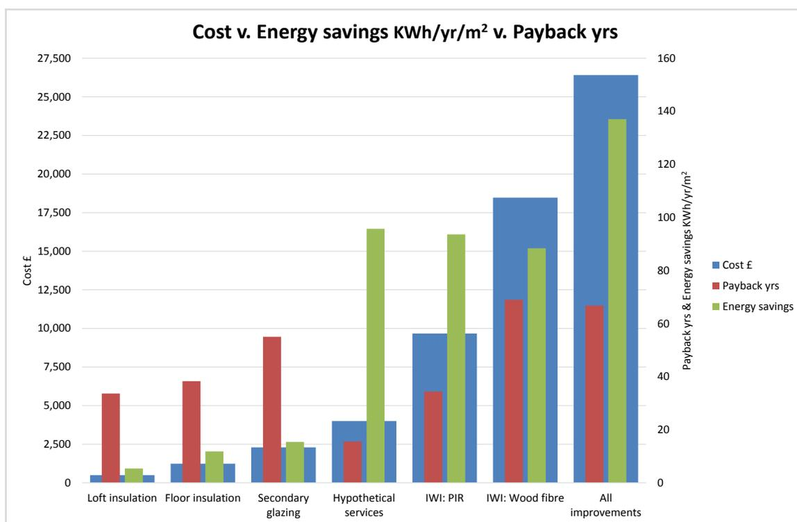
Figure 36: Comparison of cost, payback and energy savings of individual measures
