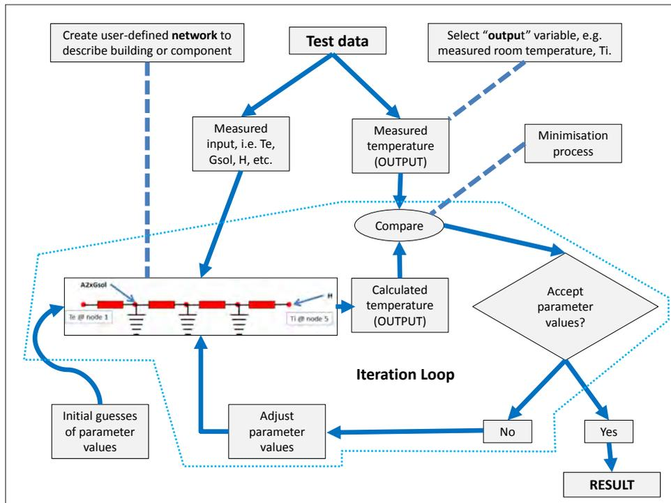
Figure A8: Parameter identification principle.
