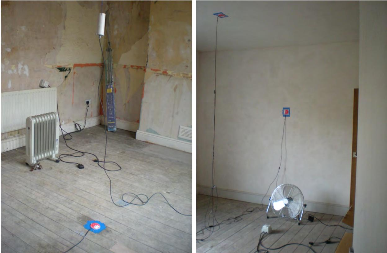
Figure 9: Co-heating test set-up with heater, fan & thermostat.
