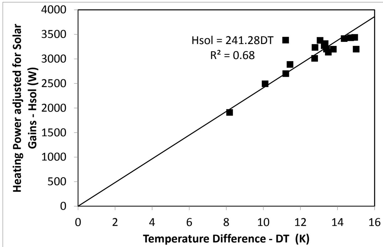
Figure A3: Example of the presentation of the data using the LMU method
