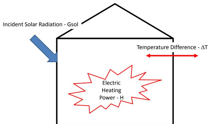
Figure 10: Schematic diagram of main parameters for analysis of co-heating test data using simplified analysis.
