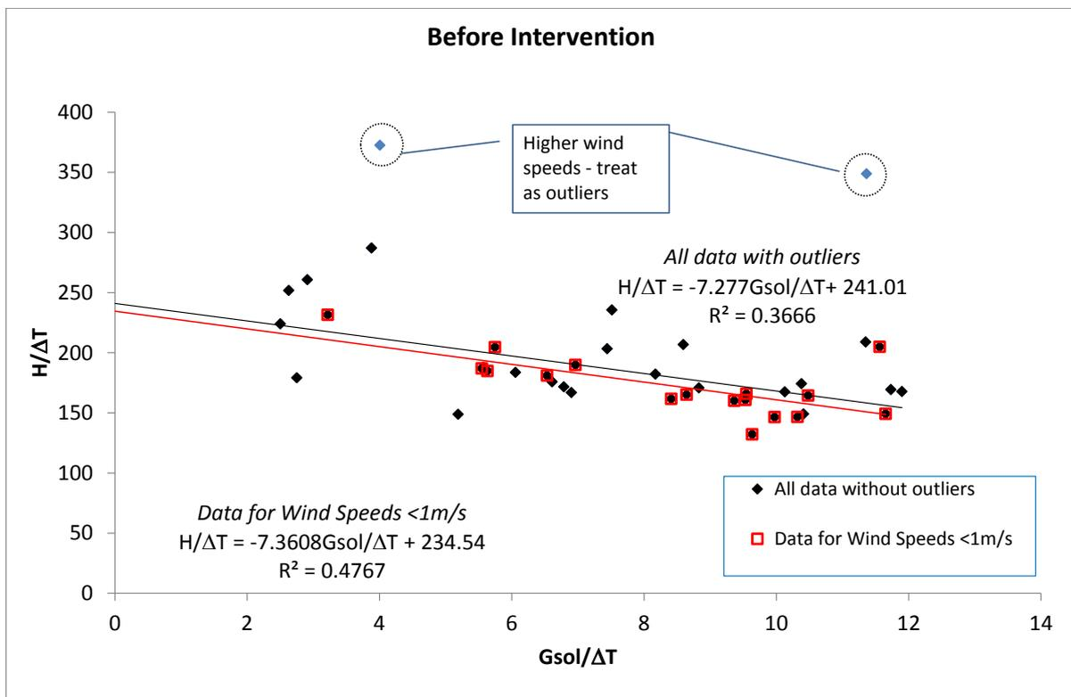
Figure A10: Before Intervention.  $H/\Delta T$  vs.  $G_{sol}/\Delta T$  plot for the daily average values from the co-heating test. The linear regression fits for all the data and only the data for wind speeds less than 1m/s are shown. The intercept on the  $H/\Delta T$  axis gives the whole house heat loss coefficient value ( $\Omega$ -value) and the slope the solar gain factor ( $gA$ -value).
