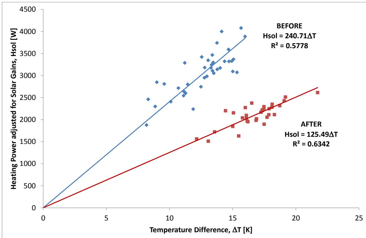
Figure A12: LMU method - heating power adjusted for solar gains plotted against temperature difference for the before and after co-heating tests.
