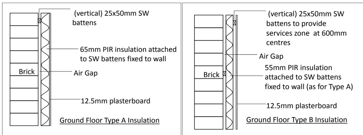
Figure 2: Ground floor insulation systems
