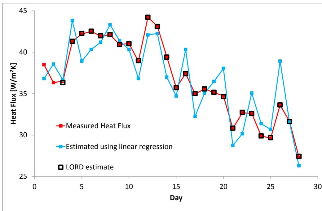
Figure A9: Comparison of the daily average heat flux estimates using linear regression and LORD with the simulated measured values for the simulated 9” brick wall. Note that the LORD estimates overlap the measured heat flux values.
