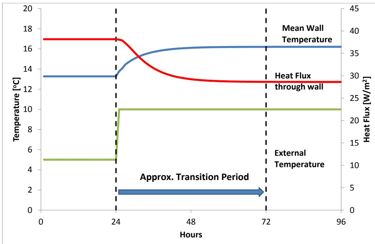
Figure A4: Simulated results for a 9” brick wall for a step change in external temperature, demonstrating the effect of thermal storage in the wall on mean wall temperature and heat flux through the wall.
