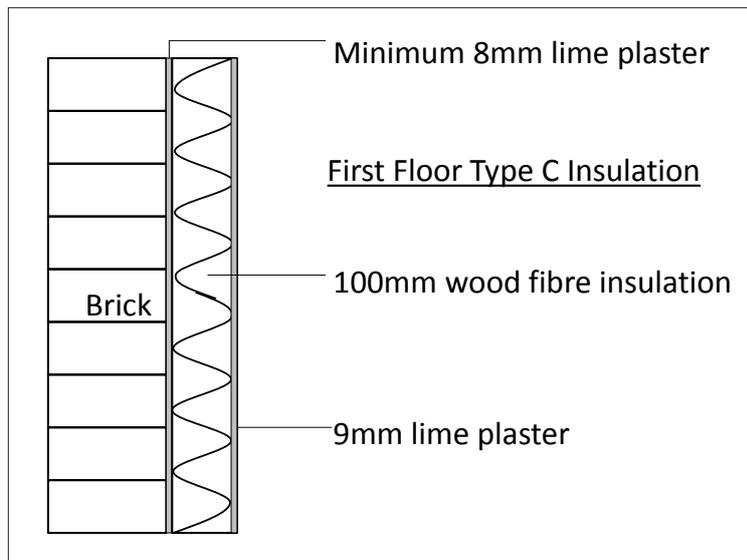
Figure 3: First floor insulation system
