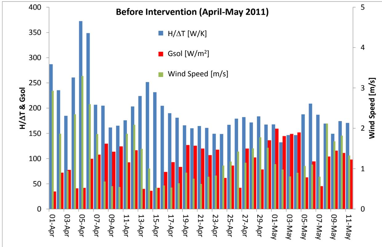
Figure 13: Before Intervention. The daily average values of H/ΔT, Gsol and wind speed during the co-heating test.
