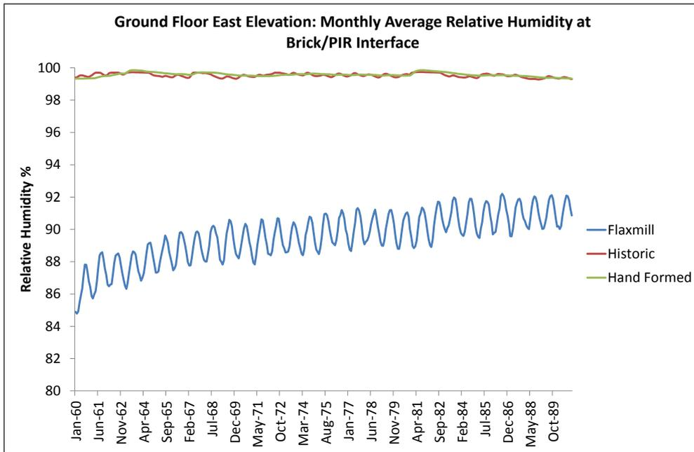
Figure 24: Ground Floor East Elevation: monthly average relative humidity at brick/PIR interface
