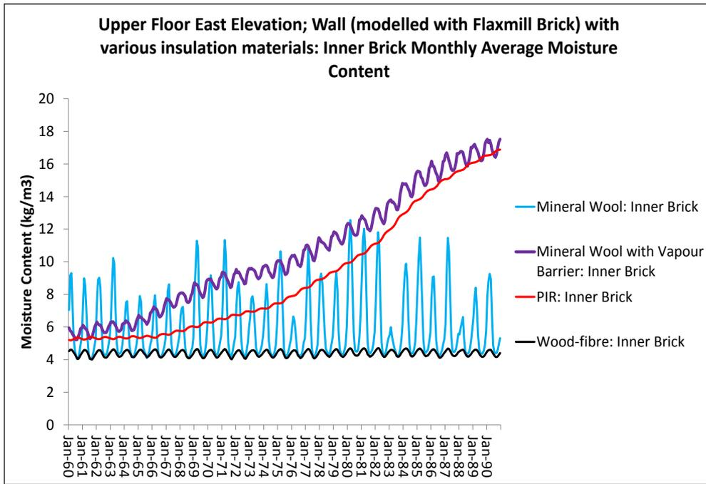
Figure 33: Upper Floor East Elevation; wall (modelled with Flaxmill brick) with various insulation materials: inner brick monthly average moisture content
