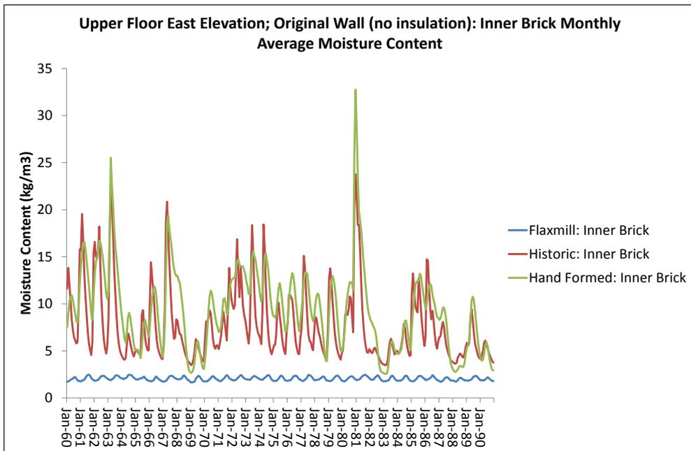
Figure 19: Upper Floor East Elevation; original wall without insulation; inner brick monthly average moisture content
