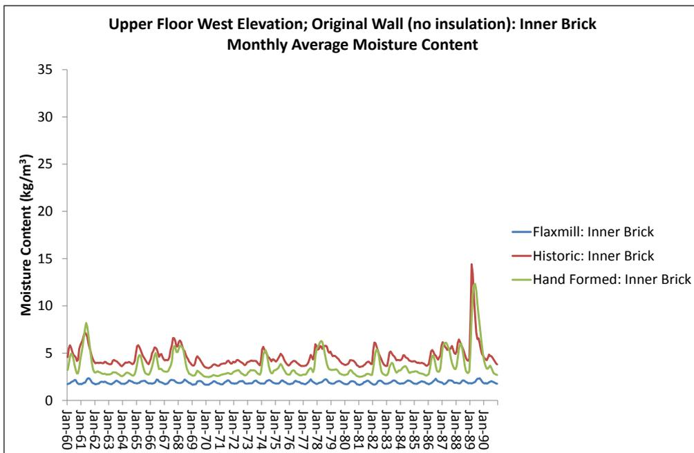
Figure 21: Upper Floor West Elevation; original wall without insulation; inner brick monthly average moisture content
