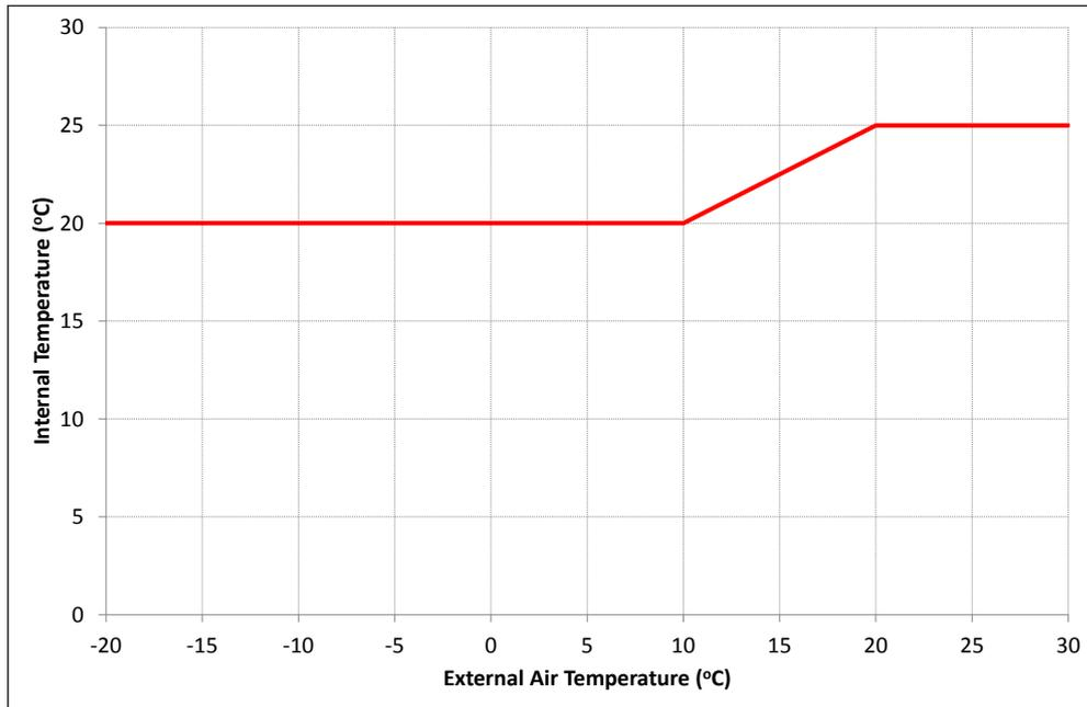
Figure 6: Variation of internal temperature with external temperature
