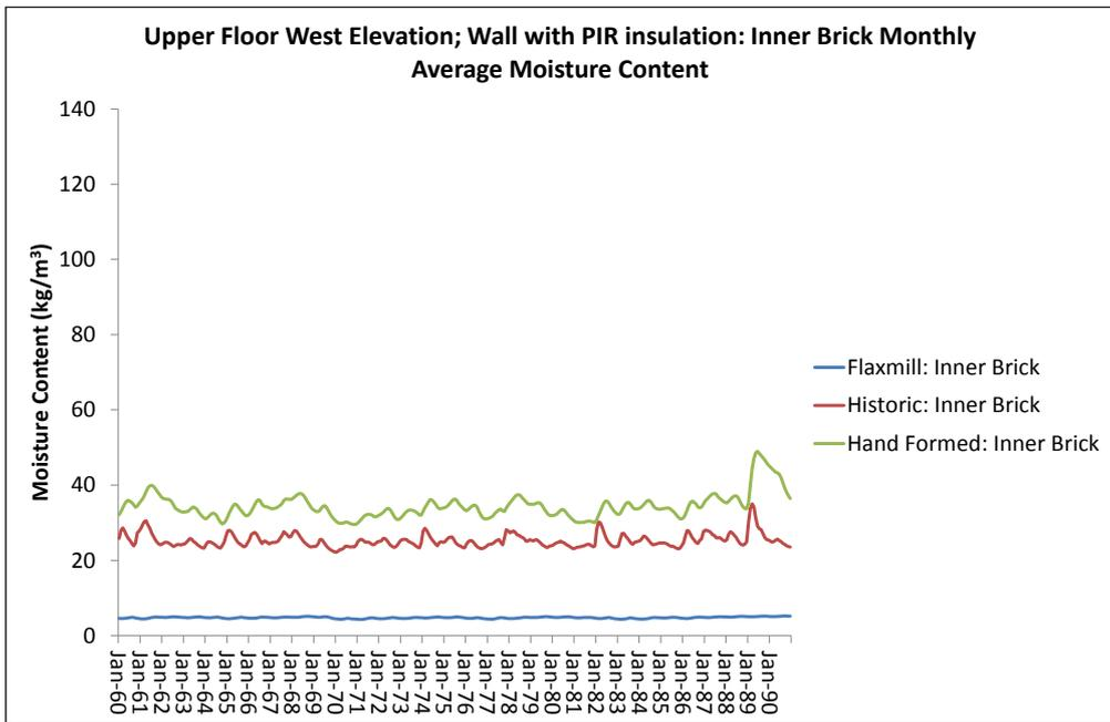
Figure 29: Upper Floor West Elevation; wall with PIR insulation; inner brick monthly average moisture content
