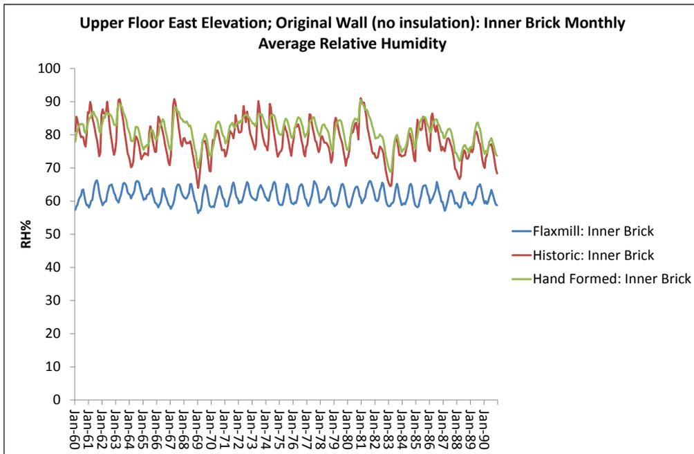
Figure 20: Upper Floor East Elevation; original wall without insulation; inner brick monthly average relative humidity
