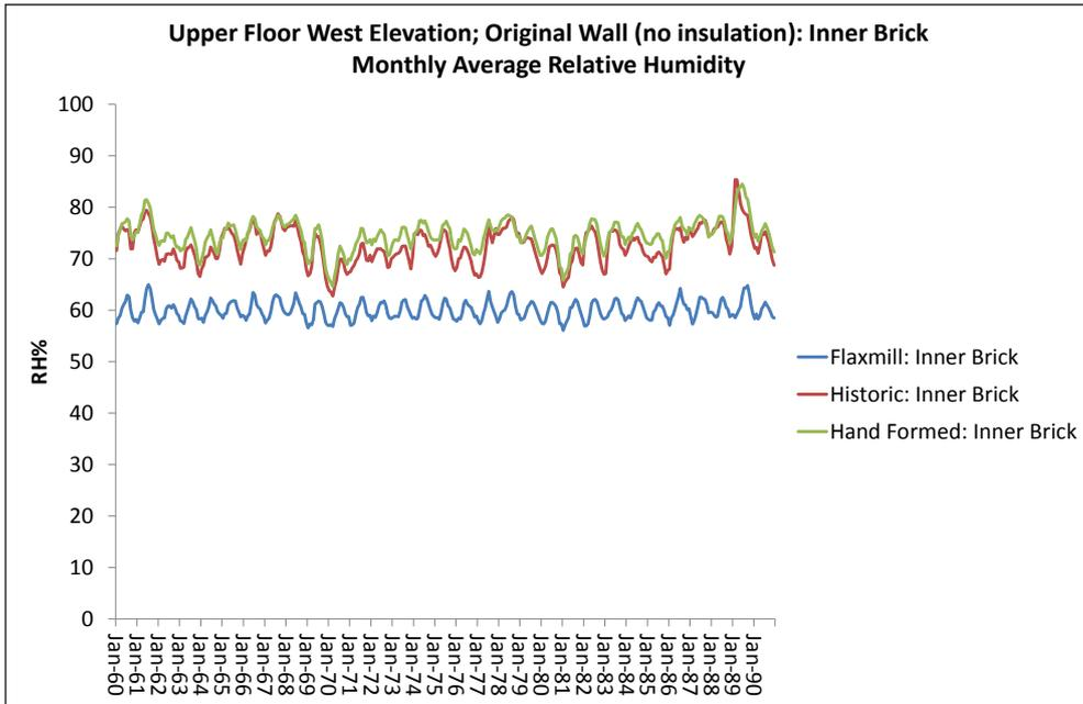
Figure 22: Upper Floor West Elevation; original wall without insulation; inner brick monthly average relative humidity
