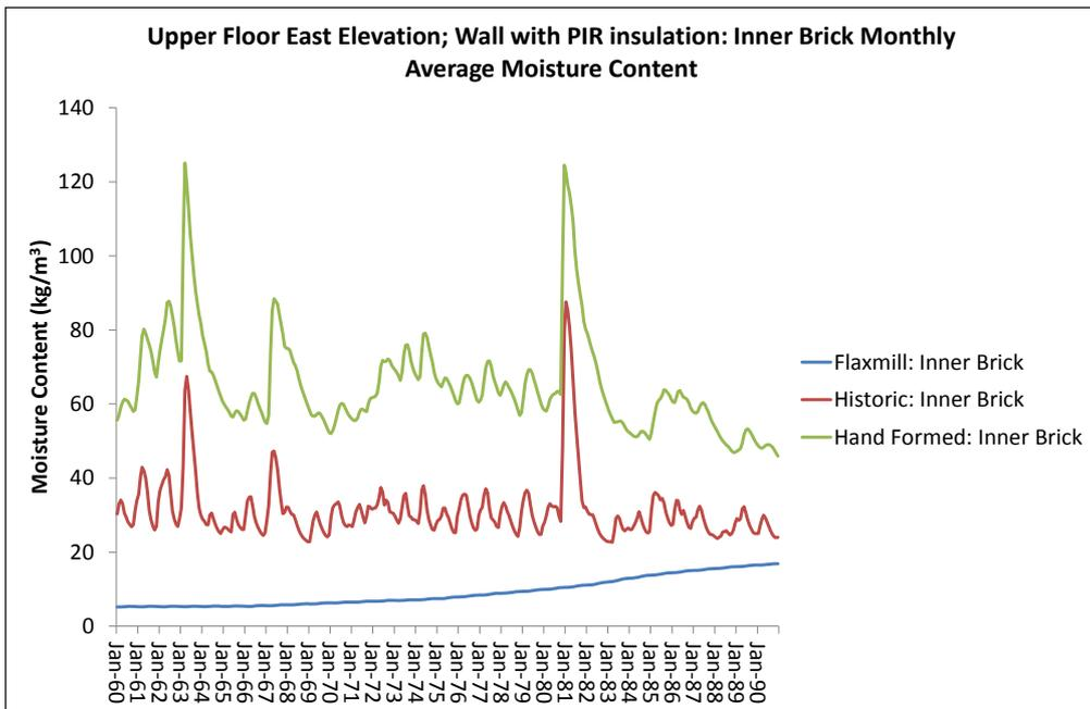
Figure 27: Upper Floor East Elevation; wall with PIR insulation; inner brick monthly average moisture content
