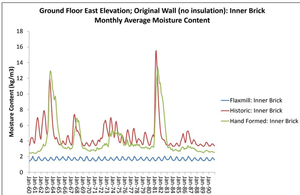
Figure 15: Ground Floor East Elevation; original wall without insulation; inner brick monthly average moisture content
