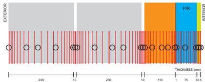
**Ground Floor, wall with PIR insulation**
