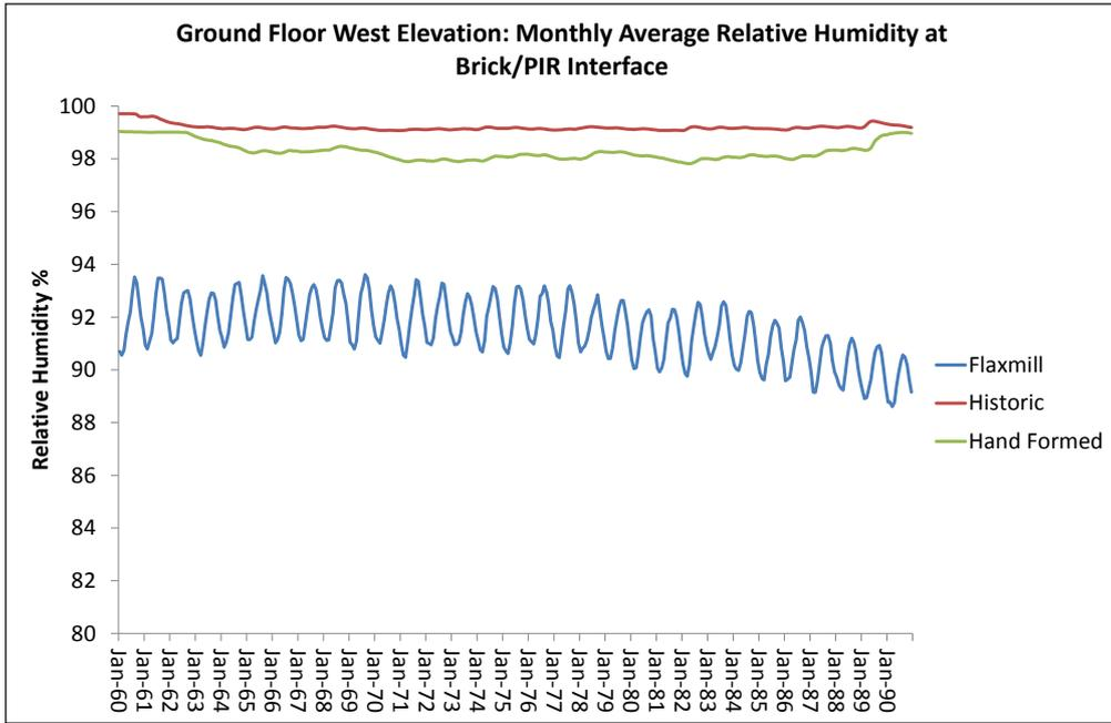
Figure 26: Ground Floor West Elevation; monthly average relative humidity at brick/PIR interface
