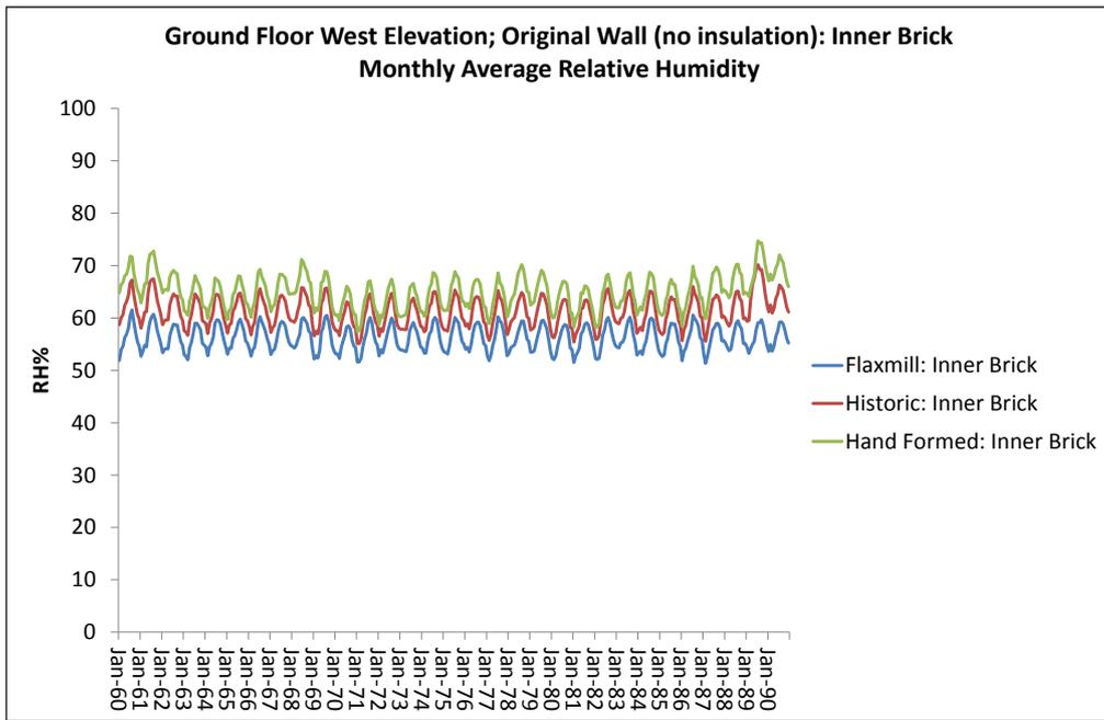
Figure 18: Ground Floor West Elevation; original wall without insulation; inner brick monthly average relative humidity
