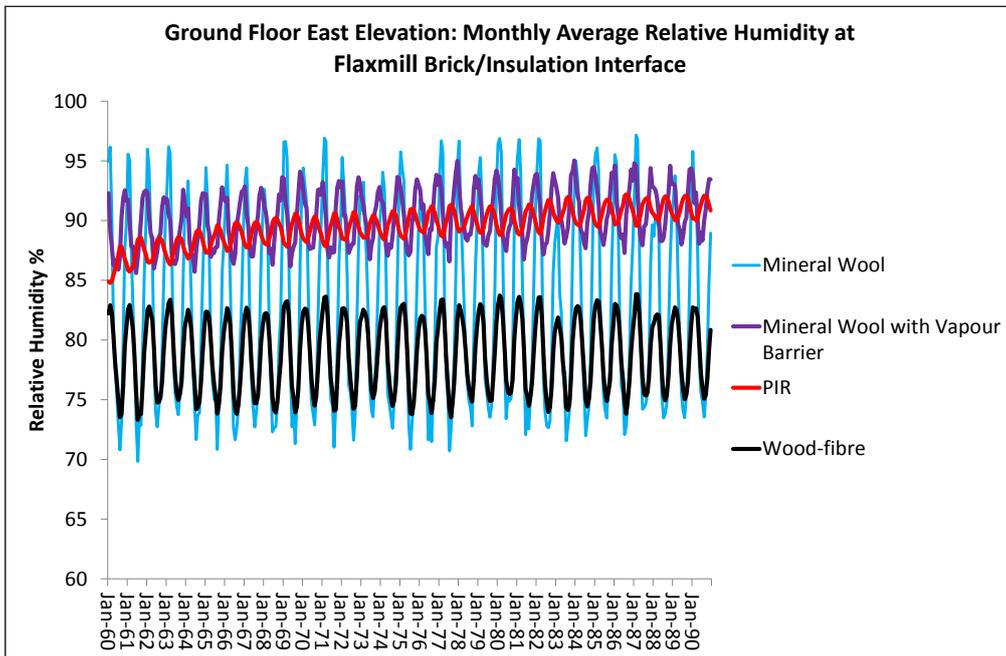
Figure 32: Ground Floor East Elevation: monthly average relative humidity at Flaxmill brick/insulation interface
