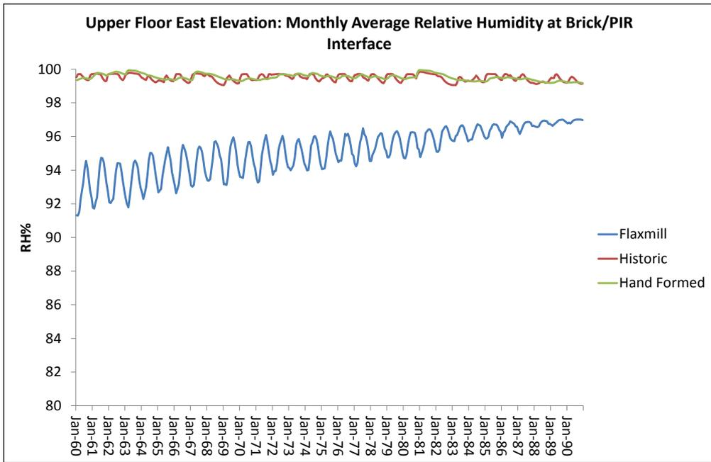
Figure 28: Upper Floor East Elevation; monthly average relative humidity at brick/PIR interface
