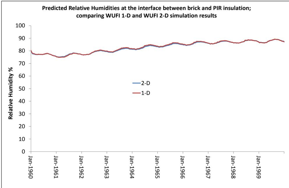
Figure 12: Comparison of 1-D and 2-D simulations of case 2 brick wall with PIR insulation
