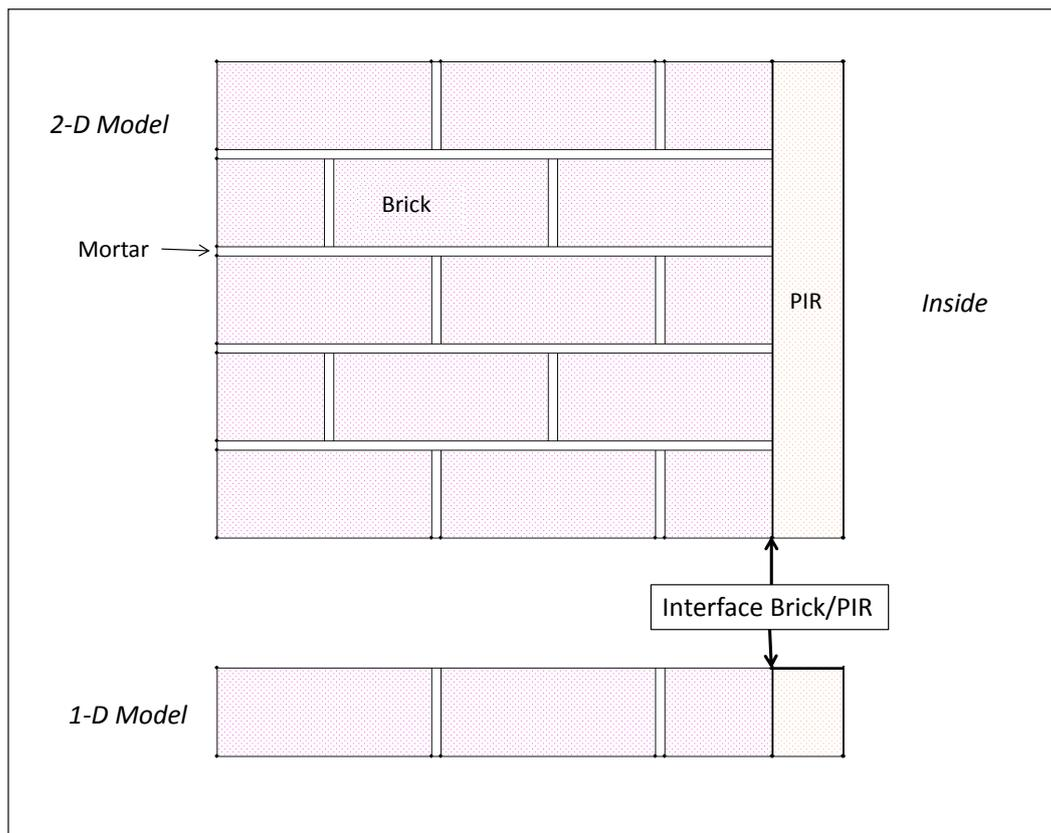
Figure 10: 1-D and 2-D models with PIR internal wall insulation
