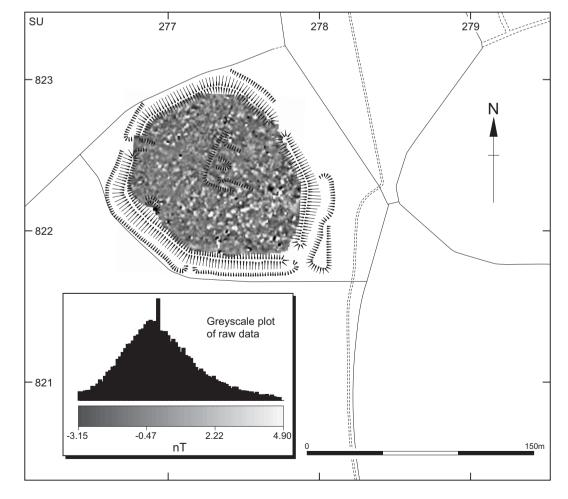
Fig 2.34 Greyscale plot of the magnetometer data from Alfred's Castle shown in relation to the plan of the hillfort earthworks.
