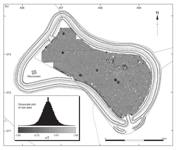
Fig 2.9 Greyscale plot of the magnetometer data from Beacon Hill in relation to the plan of the hillfort earthworks.
