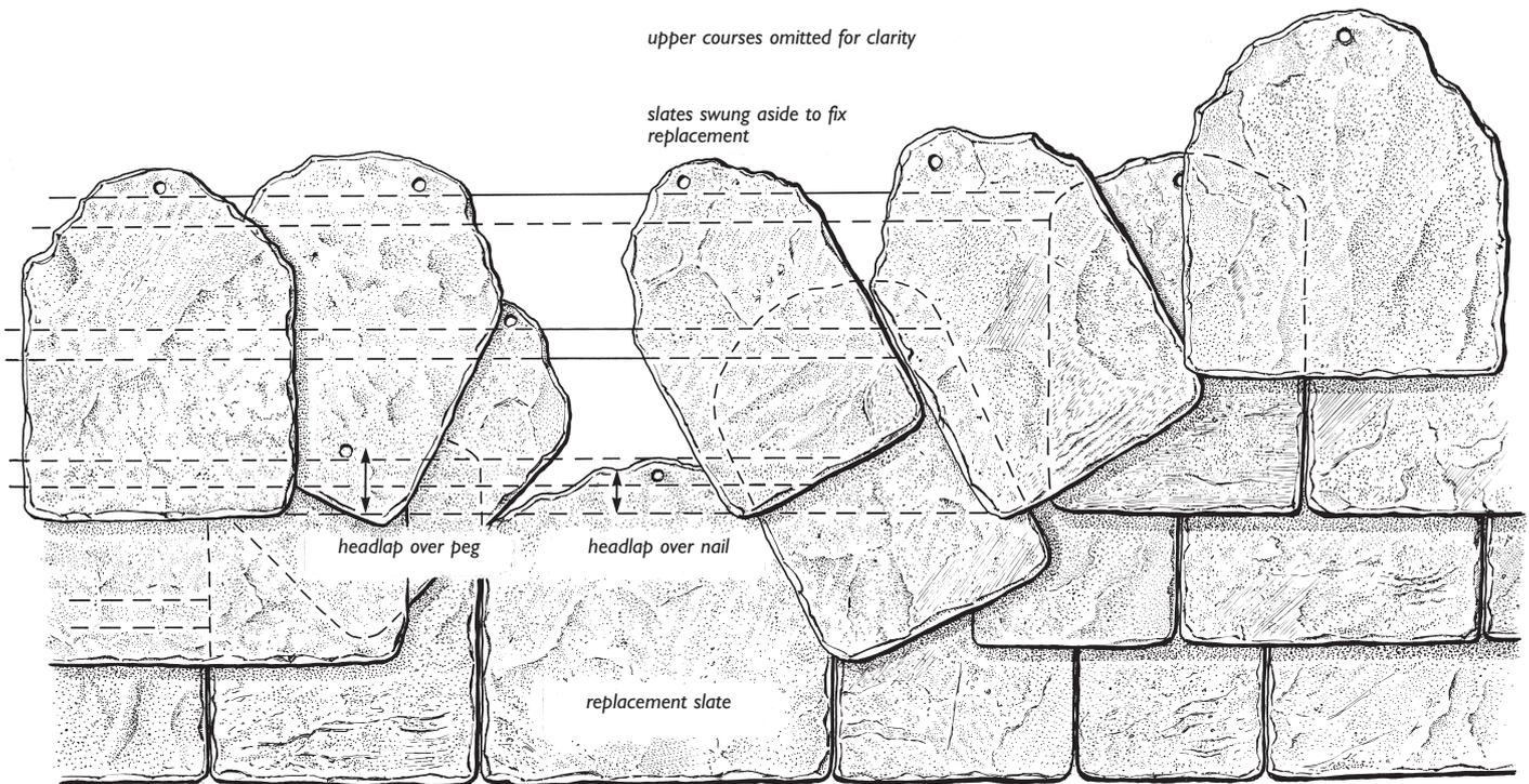
**Figure 14** Fixings for replacement slates as part of a localised repair must be aligned with the adjacent slates. If the original slates are pegged but the replacement slate is nailed, care must be taken not to compromise the minimum head lap by placing the nail too far below the pegs.
