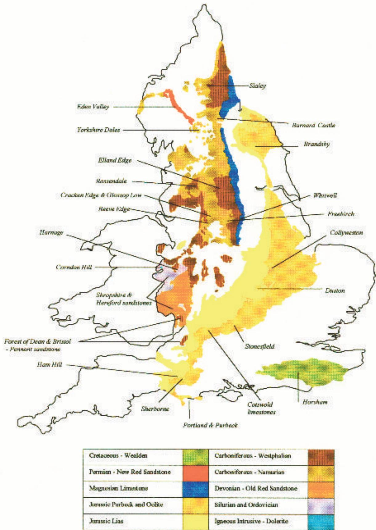
Figure 1 Geological formations important for stone slates in England, and some historical locations for production and use
