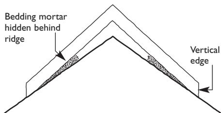
**Figure 6** The edges of the ridge should be formed as shown to avoid large and unsightly mortar fillets. Similarly ridges should not be edge pointed, rather the bedding should be neatly struck off as work progresses.
