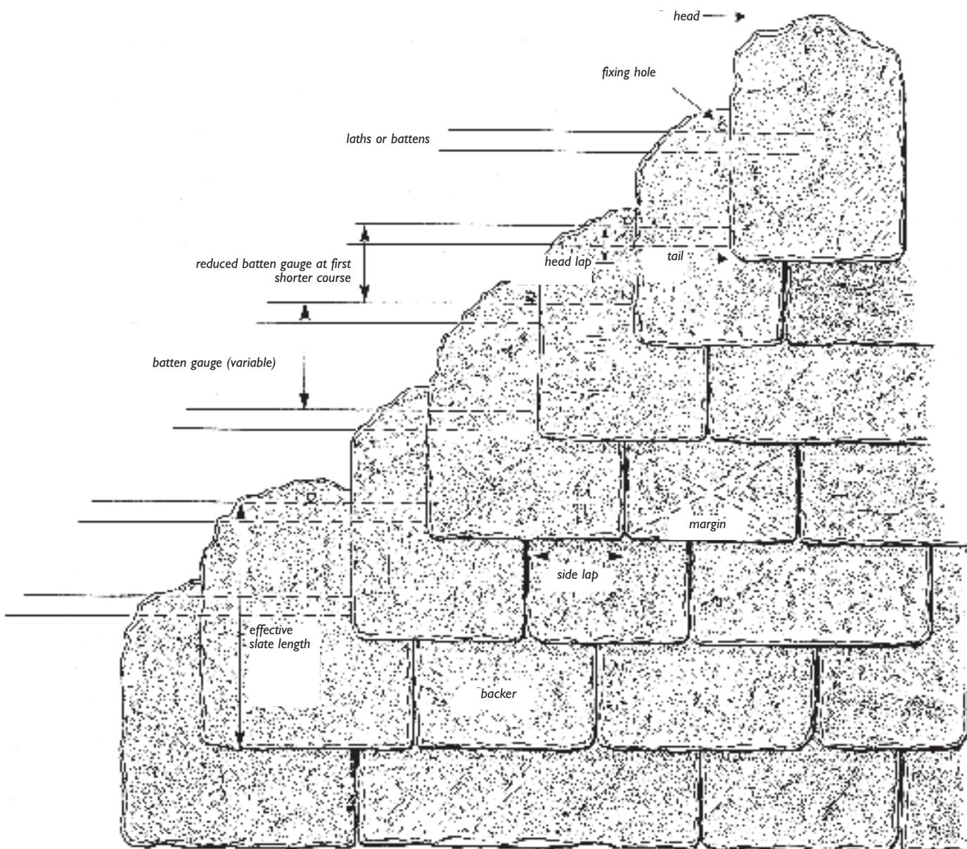
**Figure 9** Measuring slates. The length is measured from the fixing hole to the tail. The head lap is the amount by which a stone slate overlaps the fixing hole of the slate in the next course but one below.
