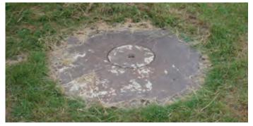
A feature sometimes associated with a forge is a wheel clamp used for putting an iron tyre onto a cart wheel. The hub is inserted into the central hole where it can be fixed with the rim of the wheel lying on the metal plate. Photo © Bob Edwards
