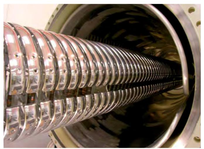
Fig 15 The power supply of the 2.5MV accelerator at Oxford open for maintenance in May 2007 (© ORAU)
