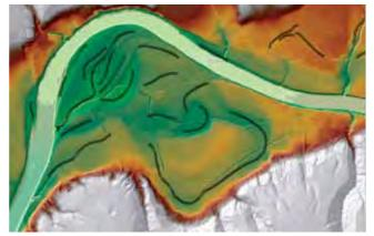
Fig 2 Palaeochannels at Osbaldeston Hall meander, lower Ribble, Lancashire shown by LiDAR (© Environment Agency)
