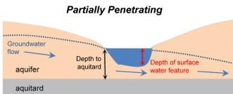
If estimated depth of surface water feature different to depth to aquitard, then feature may be considered to be fully penetrating
