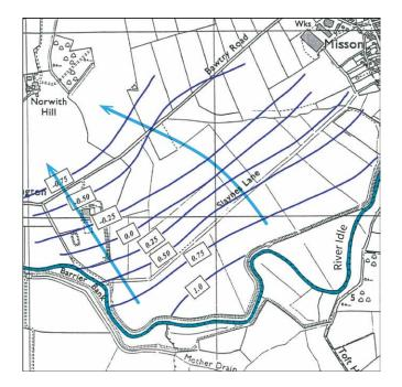
Figure 28 Sand and gravel groundwater level contours (m AOD).
