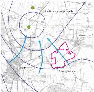
Figure 29 Sandstone groundwater level contours (m AOD).
