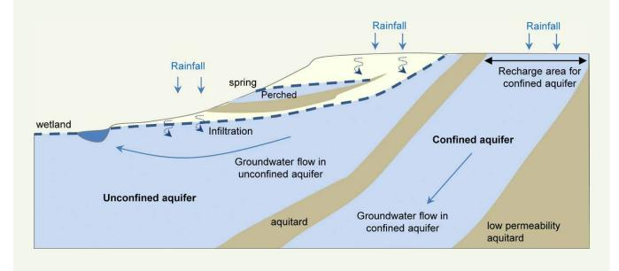
**Figure 2** Aquifer types. Groundwater levels are usually recorded with a hand-held electronic 'dip-tape' (Figure 3), with levels recorded as a depth below a fixed point of measurement, such as the top of the monitoring well. They can also be measured with *in situ* data loggers within a borehole.
