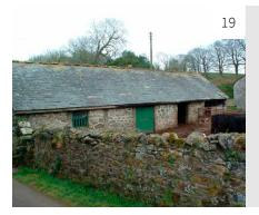
**Image 19: Pig housing** may take the form of enclosed piggeries or individual pigsties. The more common pigsties are identifiable by their small pens and yards. In areas without open yards, pigsties might be attached to or incorporated within other buildings. These are characterised by the presence of feed hatches that can be accessed from the outside.
