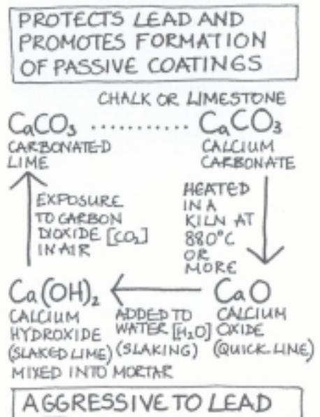
Figure 11 The lime cycle. Calcium carbonate –  $\text{CaCO}_3$  – the start and end point of the cycle, is nearly neutral, does not attack lead and can help to protect it. Slaked lime –  $\text{Ca}(\text{OH})_2$  – is alkaline and aggressive to lead.
