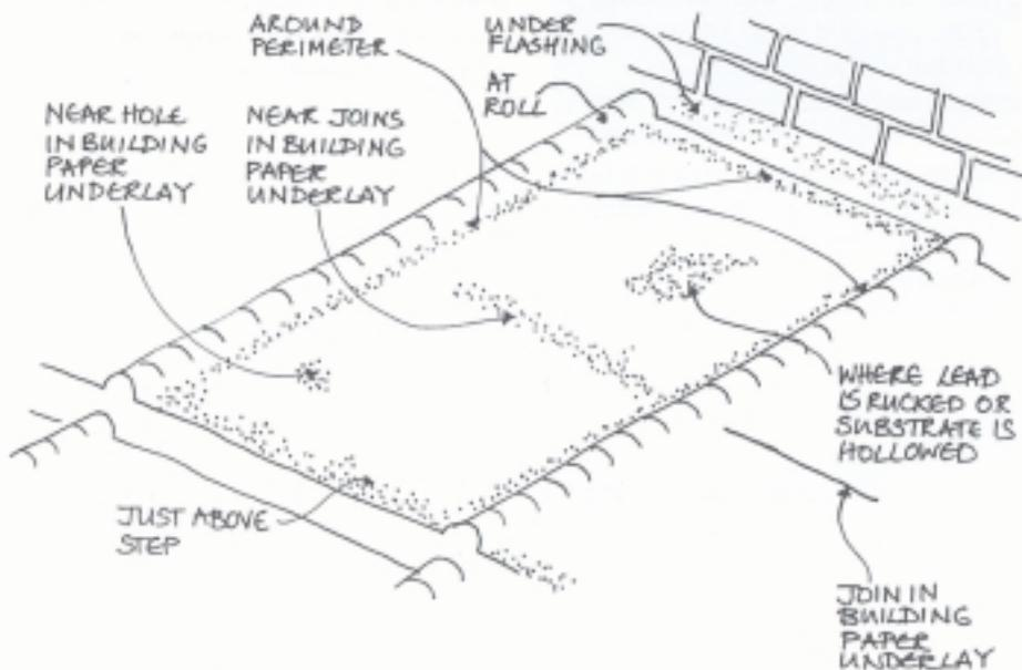
Figure 10 Typical locations of acid-related corrosion. If acids are present, corrosion is often found around the edges of the lead sheet: inside rolls, above laps, and above areas where the lead has become blistered or folded, or the substrate dips away. This appears to be a consequence of distillation of water across the air gap, easier access of carbon dioxide to regenerate acid from the lead salts, and electrochemical effects.
