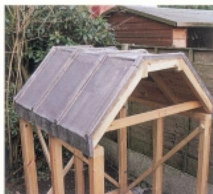
Figure 13 This outdoor test rig near Manchester has 100% outside air ventilation. Little ULC has been found here, apart from an area of the flat central section above which a shallow puddle of rainwater collects. Evaporation from this cools the lead in windy conditions (increasing the risk of condensation) and lengthens the drying-out period when it is warm. In an enclosed roof or a VWR, a small amount of moist air or water vapour entering the ventilated airspace can have a similar effect.
