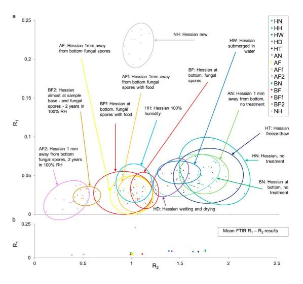
**Figure 3:** Two peak ratios for hessian fibres, termed R1 and R2 are calculated at different moisture contents and following fungal treatment: a) An R1 versus R2 plot distinguishes the different moisture and fungal treatments for at least ten specimens of hessian fibre forming distinctive clusters. b) Mean R1 and R2 values from the sample sets in part a). (Maundrill, Dams *et al.*, 2023).
