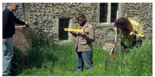
Determining relative ground levels *Top*: Interior floor levels, the difference in the interior and exterior ground levels, and the slope of the ground around the building, can all be determined to sufficient accuracy for most purposes using the simplest of tools: two straight sticks or metre rulers, a tape measure, string and a builder's level, or a line level.
