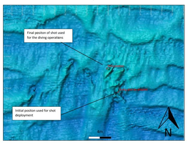
Figure 7: Position of the diving shot deployed on the Gun Site - from multibeam sonar survey (MSDS and PAS)
