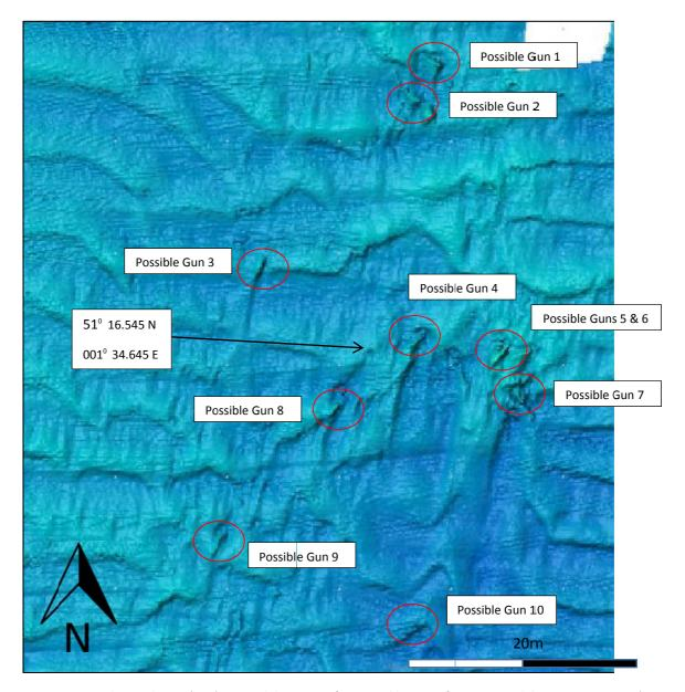
Figure 3: The North-East (Gun) site, with locations of ten possible guns - from 2017 multibeam sonar survey (MSDS W')
