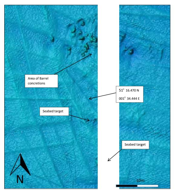
Figure 2: The North (Barrel) Site - from 2017 multibeam sonar survey (MSDS W ^)
