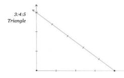
Set up a suitable baseline, and then use 30m tapes to set out a right angle using the 3:4:5 triangle method. Make the triangle as large as possible (e.g. 15:20:25 metres rather than 3:4:5 metres) as extending lines out from a small triangle is likely to be inaccurate.
