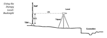
Then take a Foresight (FS) reading with the staff on the points you want to level (but never directly on a find!). The height OD of the target point (its Reduced Level or RL) is the Instrument Height minus the Foresight.
