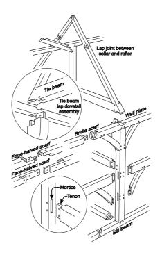
Figure 4.6 Common types of joints used in timber framed construction. After Harris, 1979, 12.
