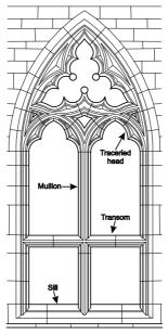
Figure 4.12 Terms for parts of a window
