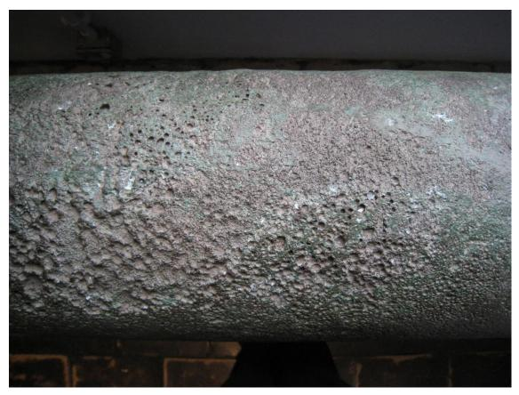
Plate 3: minor patches of active corrosion (pale areas) on Gun 1
