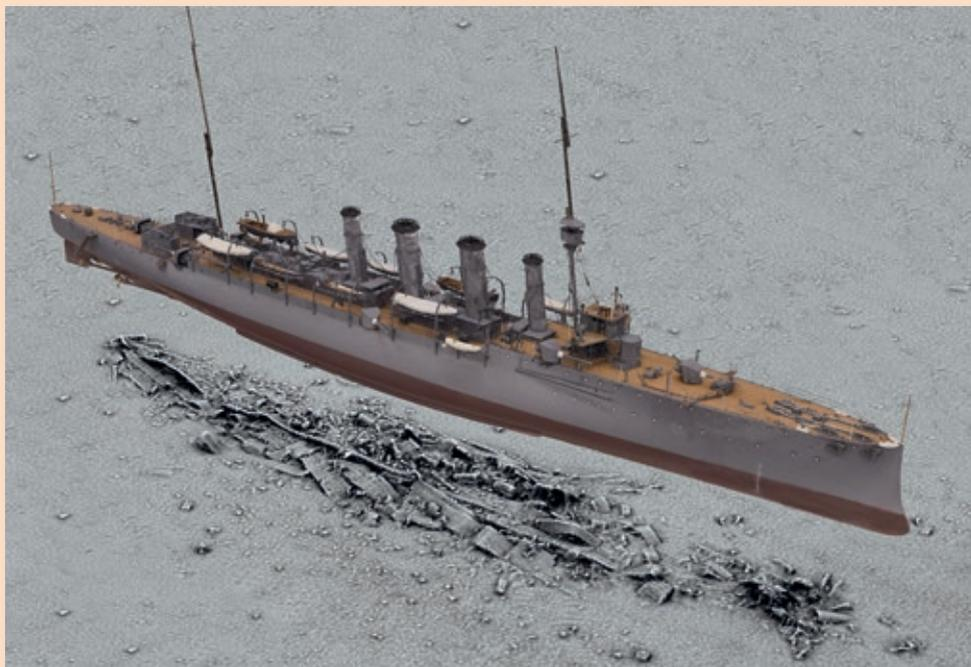
*This image shows a 3D scan of the original builder's model of HMS Falmouth in relation to a survey of the wreck on the seabed. 3D scan by Historic England. Access to ship model courtesy of Imperial War Museums. Contains Maritime and Coastguard Agency data © Crown copyright.*
