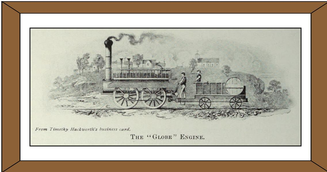
**The Globe, built by Timothy Hackworth especially for pulling passenger trains in 1829.<sup>3</sup>**
